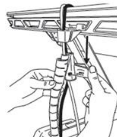
Pull down on the Cable Zip tool while holding the top of the Cable Zip.
